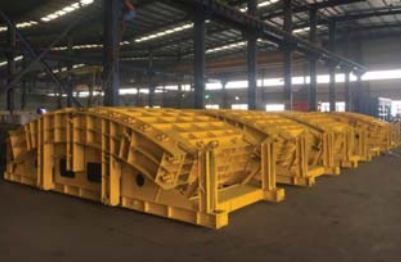
Hong Kong Dragages & Bouygues JV- TMCKL subsea tunnel tunnel D17m - Foldable 2 stages covers with spring
