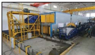
Double layers of Steam curing Chambers for China, Shanghai CCC
