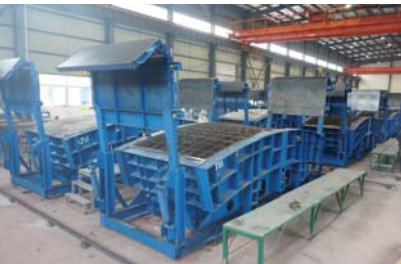
Hong Kong Dragages & Bouygues JV- TMCKL subsea tunnel tunnel D17m - Foldable 2 stages covers with spring
