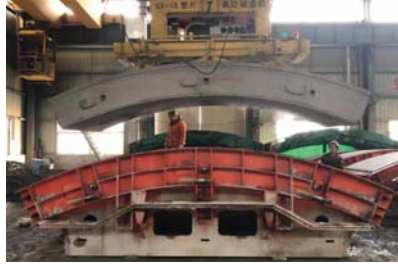
Japan Ando-Hazama Road tunnel D12.4m - Casting cover + sliding open for mould panels+ Vibration table
