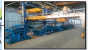
Semi-Auto Segment production line with Vibration table for Vietnam HoChiMinh City Metro
