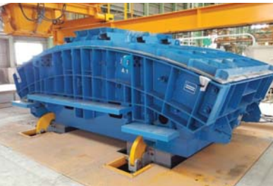
Japan Ando-Hazama Road tunnel D12.4m - Casting cover + sliding open for mould panels+ Vibration table
