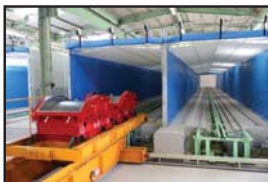
Japan-Carrousel for segment production: Nippon Hume Concrete factory.
